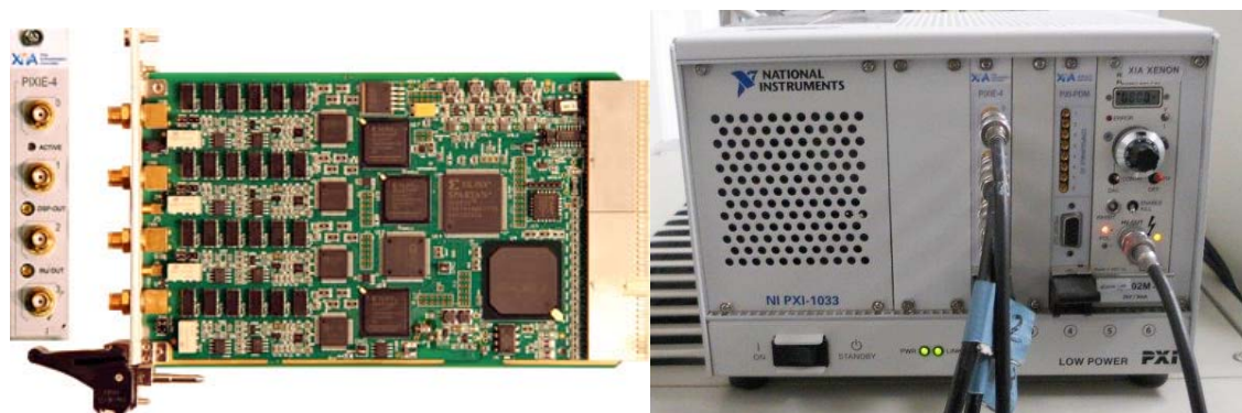
Fig. 4 Pixie-4 and PXI electronics configuration
