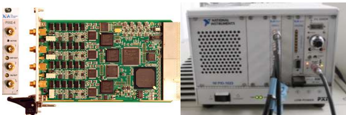
Fig. 4. Pixie-4 and PXI Electronics Configuration.
